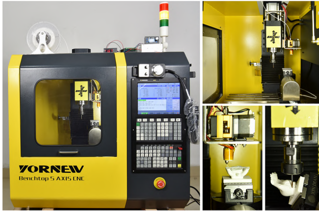
Fig. 19. Our ASHM machine was modified from a CNC machine (YORNEW Benchtop 5 Axis CNC MX220). The accessories of the additive module are installed above the machine (left). The additive extrusion module is connected with the machine spindle in parallel (upper right). The lower right corner demonstrates the additive process and subtractive process.
