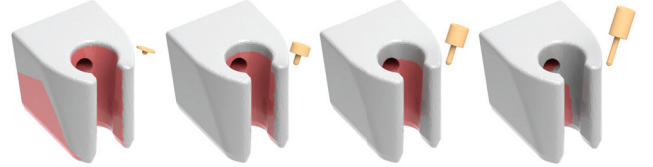
Fig. 11. Illustration of the effect of cutter length on inaccessible regions. Generally, longer cutters lead to fewer inaccessible regions.
