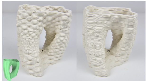
Fig. 22. The Julia vase model was decomposed into four OPPs with different textures.
