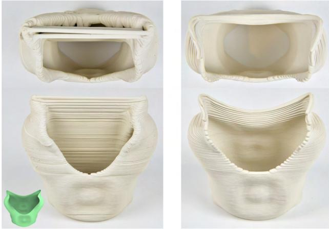
Fig. 2. Left: a strictly-continuous path generated by [Hergel et al. 2019]. We tailor this method to surface models by slightly thickening the original surface into a model with a valid volume. However, the redundant non-model structure still needs to be used to connect separate components of the model (see the top view). Right: Our toolpath is fully continuous due to the use of curved layers, without requiring an extra path.
