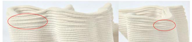
Fig. 19. The thickness was non-uniform in the outer boundary of the curved layers because the material deformed in different ways when extruded in the downhill or uphill directions.
